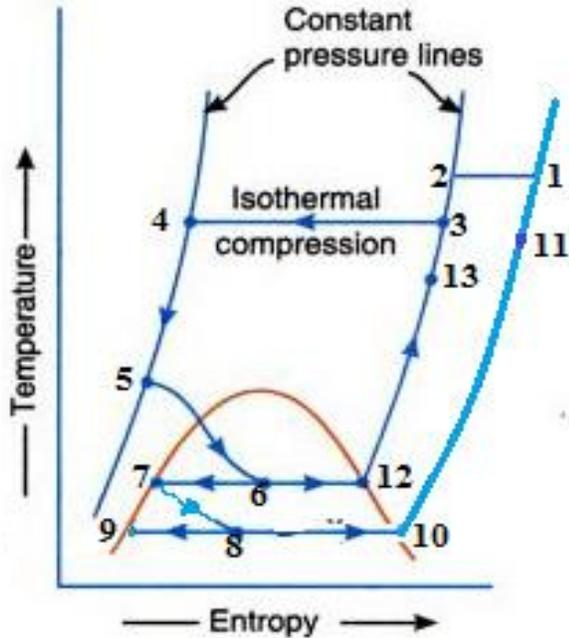
Figure 1(b): T-S diagram of Dual compressor Linde system
